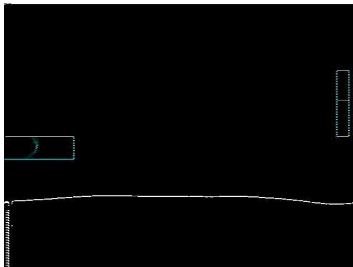
Figure 45: Illustration of output of Non-Maximum Suppression followed by Hough Transform Overlay
